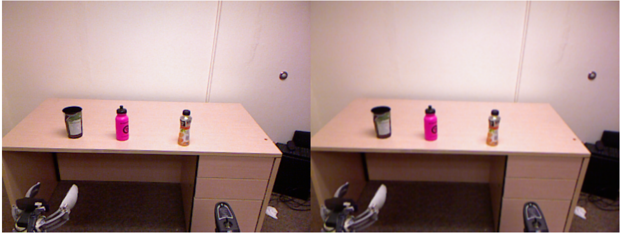
Figure 4.5: Output after noise filtering. The image on the left shows the source image and the image on the right shows the output after noise filtering.
